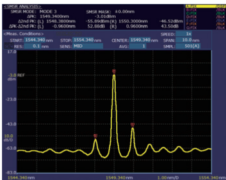
The side mode suppression ratio (SMSR) of laser can be measured quickly and accurately.
