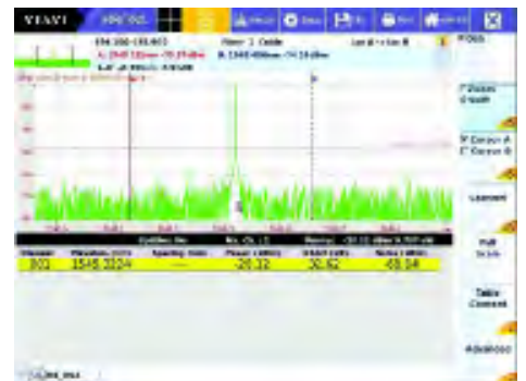
Wavemeter GUI with tabulated wavelengths, powers, and low-resolution graph
