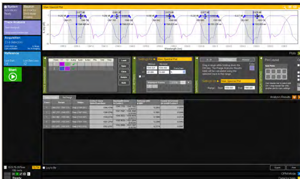
Figure 2. Example of mSWS interleaver scan
