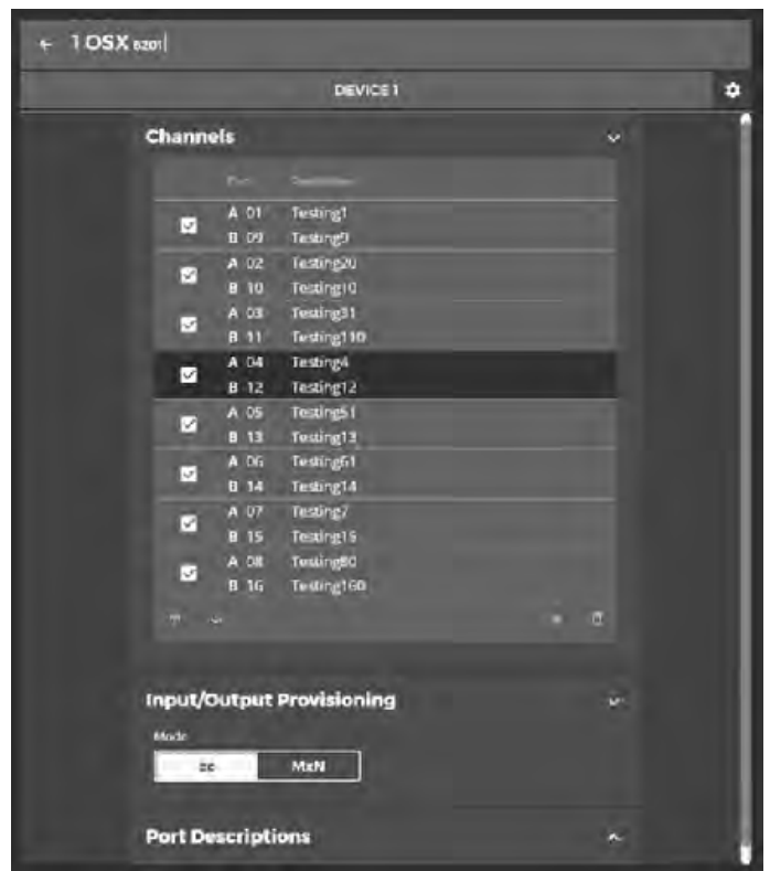
Figure 4. mOSX-C1 MAP-300 summary view with port labels. Active paths shown with check box
