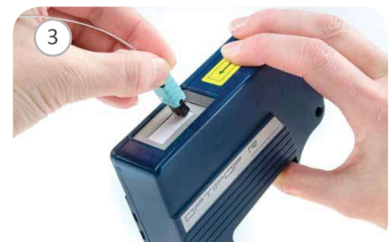
3 Place the connector on the wet area of the cloth and wipe from the wet area to the dry area
