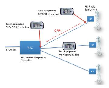
CPRI Layer 2 testing includes REC or RE emulation, BER traffic generation, control words decode and frame capture capabilities to troubleshoot interoperability, transport or RF performance issues.
