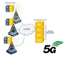
To ensure that 5G network's strict requirements are met in the fronthaul, the eCPRI Transport Network requirement document establishes classes of service for data and C&M traffic. With full line rate eCPRI traffic generation capabilities and high accuracy one-way latency measurements, the RXT6200 provides the tools necessary to ensure that the eCPRI transport network is ready for 5G deployments.
