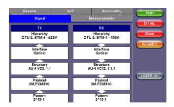
The transmitter and receiver can be set up independently, or coupled depending on the application. Framed signals can be equipped with unstructured or structured payloads with selected test pattern filling the entire test payload (Bulk) or a structured payload (SDH/SONET framed client signal) with or without PDH/DSn multiplexed clients. The test payload can be sent in one channel only or broadcasted to fill the entire link.
