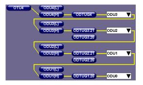
OTU4 Single-step mapping/multiplex structures
